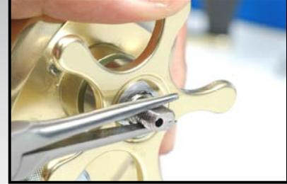
With the click pin held in place by the star drag washer, spin the star drag onto drive shaft. Use pliers to hold the shaft from spinning.
