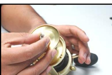
Reinstall spool and side plate. General maintenance is now complete. For further maintenance on reels that have had extensive usage, or excessive exposure to saltwater, please refer to the next page.
