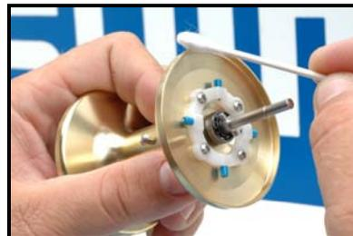
Inspect and clean spool assembly. It is highly recommended that fishing line (especially braided line) be removed from the spool at least once a year to prevent spool corrosion.
