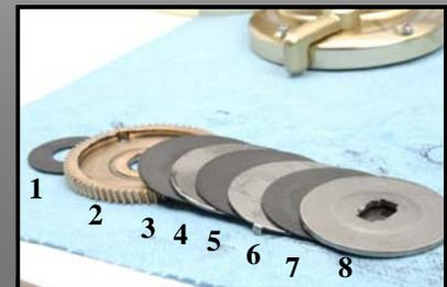
It is good practice to lay drag washers out in sequence in order to facilitate easy reassembly.
