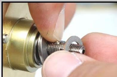
To reinstall click pin, push click pin down and use the star drag washer to hold the click pin in place.
