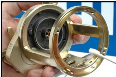
Clean exterior of reel with isopropyl rubbing alcohol and cotton swabs or toothbrush. Shimano® Bantam™ Oil may be used on the reel foot to prevent corrosion.
