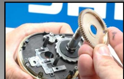
Reinstall drag washers and drive gear.
